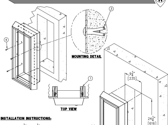
A. PROVIDE  $9\frac{1}{4}$ " X  $24\frac{1}{4}$ " WALL OPENING AND BACKING (1) TO ACCEPT CABINET. MINIMUM  $3\frac{1}{4}$ " DEPTH FROM FINISHED WALL.
